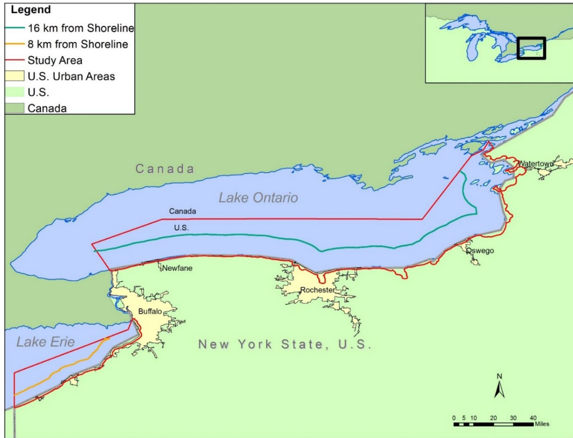
Figure S-1. Study Area with 16 km (10 mi) Line in Lake Ontario and 8 km (5 mi) Line in Lake Erie Indicating the Offshore Turbine Zones and Inshore Cabling Zones for Each Lake
